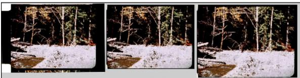
Process of Rectifying a frame scan. Left is the frame scan, with overscan into the frames above and below. Center is the frame, cropped to exact pulldown (image area plus one frame dividing line). Right, the frame is now re-scaled to 3000 pixels high, so the scan now has a rectified scale of 1 pixel equals 0.0001\*, compared to a 0.3000" standard 16mm film pulldown.
